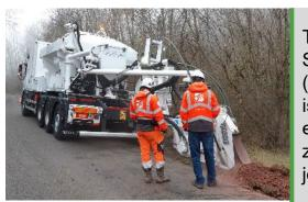
The evolution of the SC4P to the E-Sidecut (a fully electric trencher) is a demonstration of an electrification path to zero-emission urban jobs.
