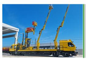
Egypt - "Green Line" High Speed Rail: Supply of 2 units model OCPD001, part of the innovative "working train" made of 6 rail vehicles to electrify a new double railway line of 660 km.
