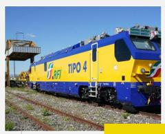
Diagnostic vehicle TIPO 4 in the RFI fleet, marking a milestone in the deployment of nextgeneration diagnostic solutions
